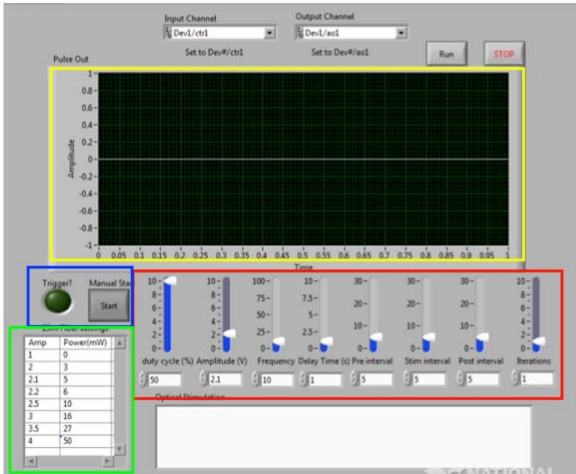
Figure 41: Screenshot of user interface of optical stimulator controller. Yellow box: Graph of optical stimulation pattern. Red box: Stimulation parameter controls. Blue box: MR scanner synchronization monitor. Green box: Calibrated settings for optical power output.
